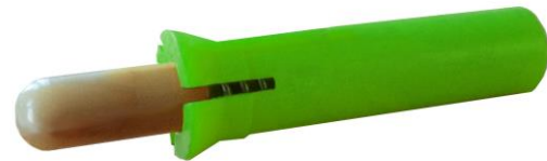
Picture 1 Spring loaded plunger used in the gear shifter
