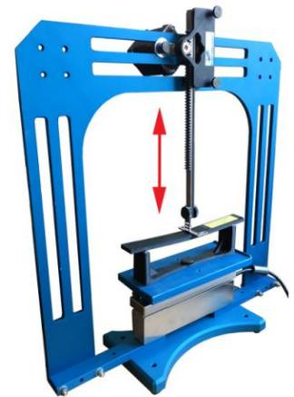
The ForceBoard Multisystem fatigue testing feature can subject test samples both to a set displacement or to a set force. Both the standard and tensile testing versions of [ForceBoard Analyzer](#) are included when you buy a MultiSystem.
