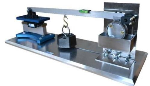
**D - ForceBoard™ Tactile Tester:** World unique **haptic perception** and tactile friction tester with built in finger position tracking and full 2D force sensing. Link your test data to subjective sensations and optimize your product!
