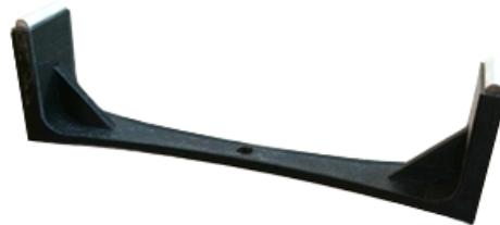
3 point bend fixture for flexural modulus testing
